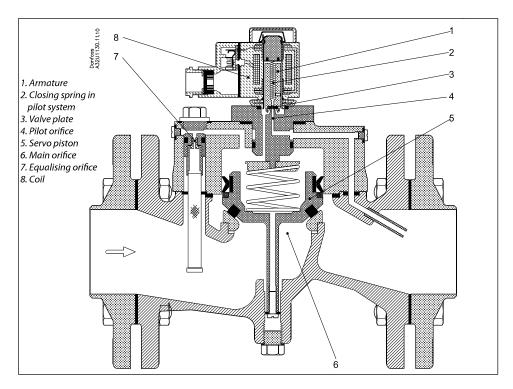
Coil voltage disconnected (closed):
